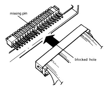
Make sure the holes fit over all the pins and then push in the connector.
